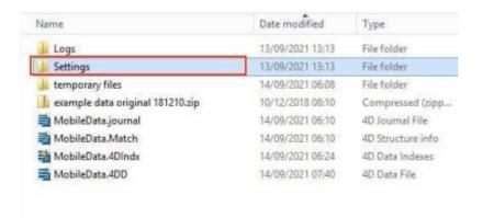
Above, note that the Settings folder is next to the mSupply data. This setup allows for the mSupply server to be updgraded with backup and memory settings intact.
