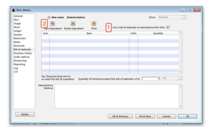
Here you can specify a Bill of Materials for the item if it is a manufactured item. Once you have done so, and have checked the **Use a Bill of Materials to manufacture this item** check box, when you enter a new build, it can be automatically filled out with the correct materials (ingredients) and the correct quantities for the total to be manufactured.
