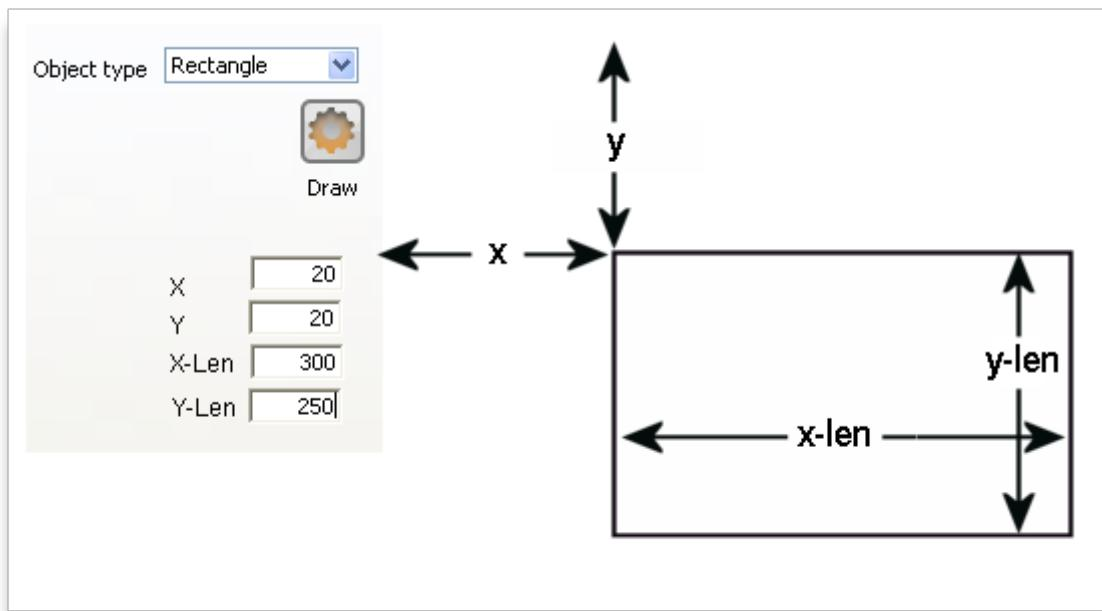
So, as an example, the coordinates are entered as above in the appropriate boxes, then the *Draw* button is clicked to produce the following display under the layout tab:
