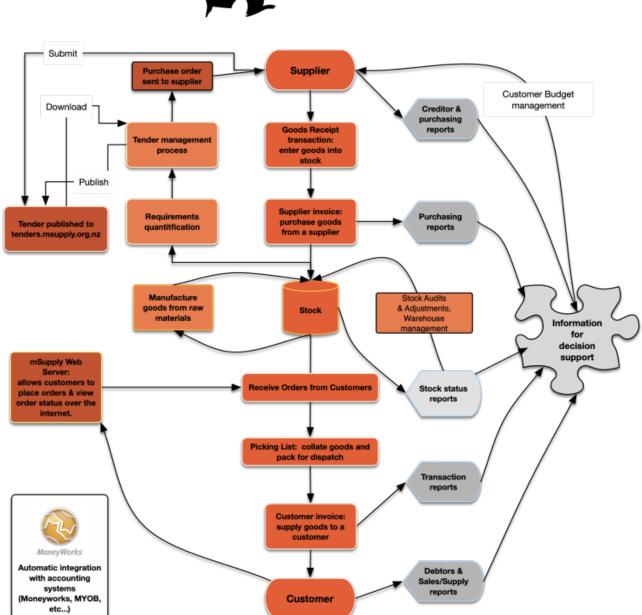
The two most common transaction types in mSupply are the **supplier invoice (si)** and the **customer invoice (ci)**. These transactions record stock purchases from suppliers, and stock supplies to customers respectively. mSupply records stock adjustments through these two transactions. So, given an opening balance of stock, mSupply will show a series of transactions that result in the recorded closing stock.
