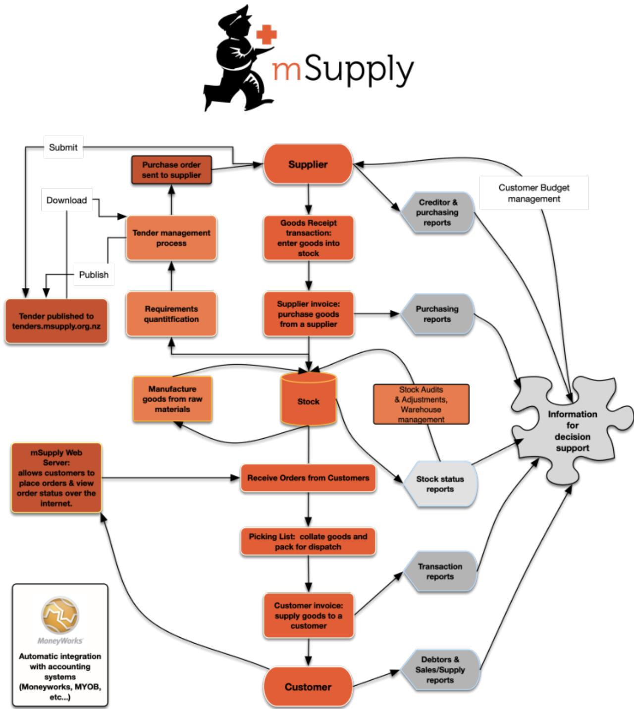
The two most common transaction types in mSupply are the **supplier invoice (si)** and the **customer invoice (ci)**. These transactions record stock purchases from suppliers, and stock supplies to customers respectively. mSupply records stock adjustments through these two transactions. So, given an opening balance of stock, mSupply will show a series of transactions that result in the recorded closing stock.
