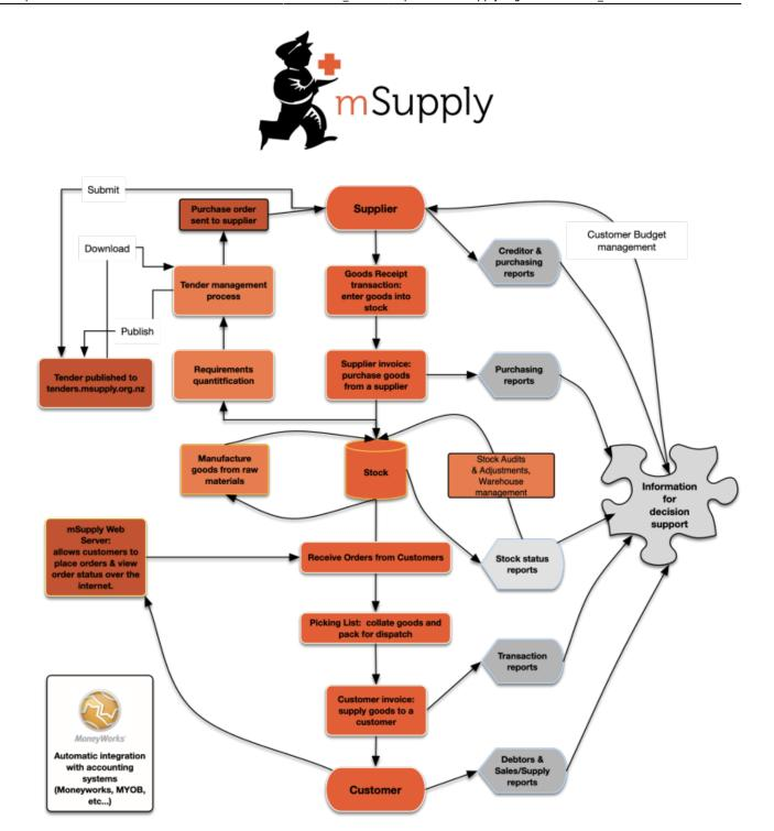
The two most common transaction types in mSupply® are the **supplier invoice** (si) and the **customer invoice** (ci). These transactions record stock purchases from suppliers, and stock supplies to customers. mSupply® records a full audit trail by only allowing stock adjustments by way of a transaction. Therefore, given an opening balance of stock for the year, mSupply® can show a series of transactions that result in the recorded closing stock.
